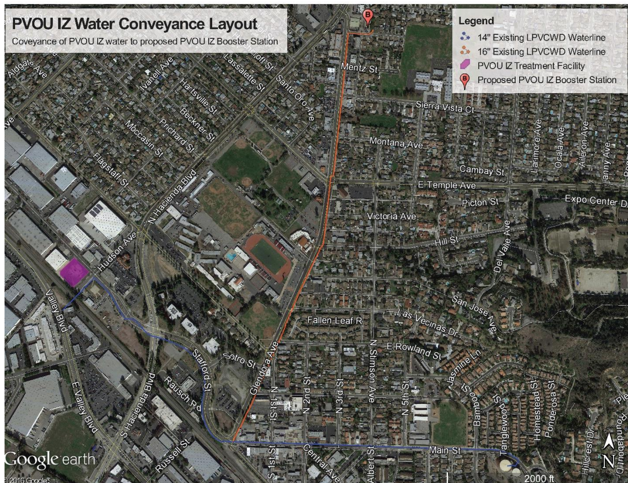
Figure 1 – PVOU IZ Water Conveyance to Proposed PVOU IZ Booster Station
