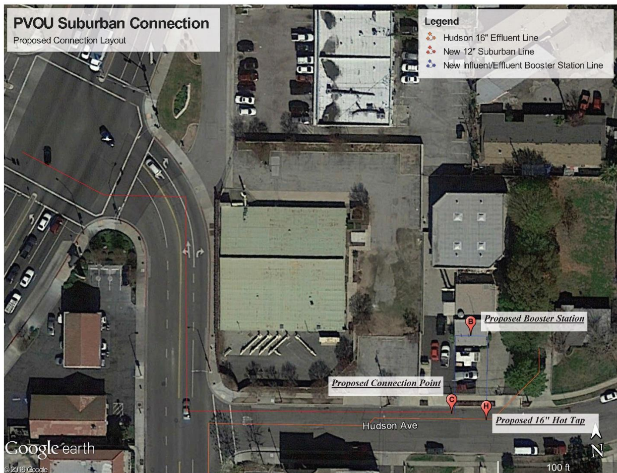
Figure 2 – Interconnection of PVOU IZ Water to SWS
