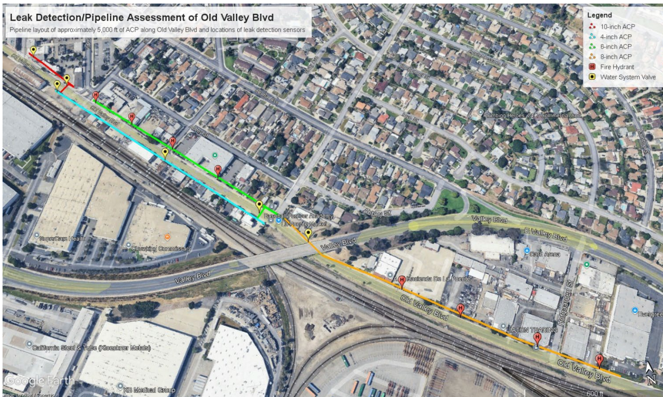
Figure 1 – Leak Detection/Pipeline Assessment of Old Valley Blvd
